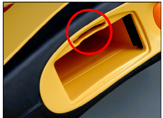
Figure 2 – Verify there is no data card installed in the card slot. If there is a data card installed, remove the data card by pushing the card in and releasing. The card will partially eject and can then be removed.
